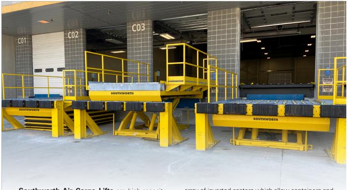
**Southworth Air Cargo Lifts** are high-capacity, heavy-duty scissor lifts designed to raise, lower and maneuver large, heavy Air Cargo Containers / Unit Load Devices (ULDs). Standard units boast a 15,000 pound capacity (higher capacities available) and platform sizes up to 13' x 13'. The platform deck is coated with a grit finish and is equipped with a grid
